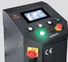
HMI control panel, portable and recharged wirelessly
