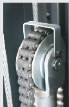
Chain support with derailment protection
