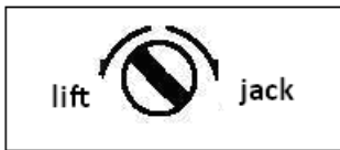
Transfer-switch 1 on the control panel
