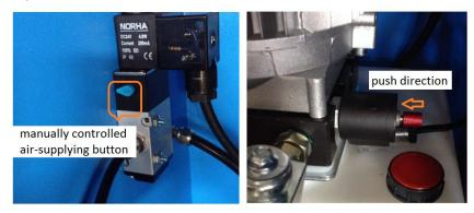
4. Turn off the unloading valve by pushing and turning clockwise the red spool until hear the sound which implicate the valve is closed. **NOTE:** For different models, the pictures showing above may differ from lift to lift, but the methods is the same.
