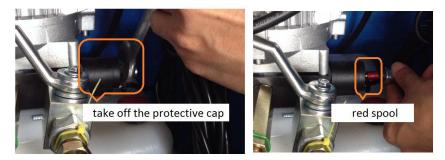
3. Push the blue air-supplying button and meanwhile push and turn anticlockwise the red spool until hear sound which implicate the valve is open. At this time, lifting platforms may lower.
