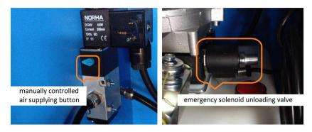
2. Take off the protective cap of the valve and see red spool of the valve.
